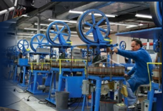
Metal and fabric cable harness overbraiding facility
