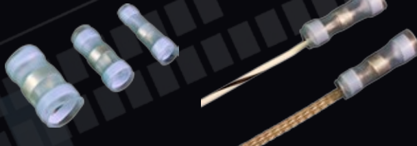
Wired and unwired AS83519/1 and /2 Type heat shrink terminations for EMI shield-to-ground termination applications (note braided versions qualified for lightning strike)
