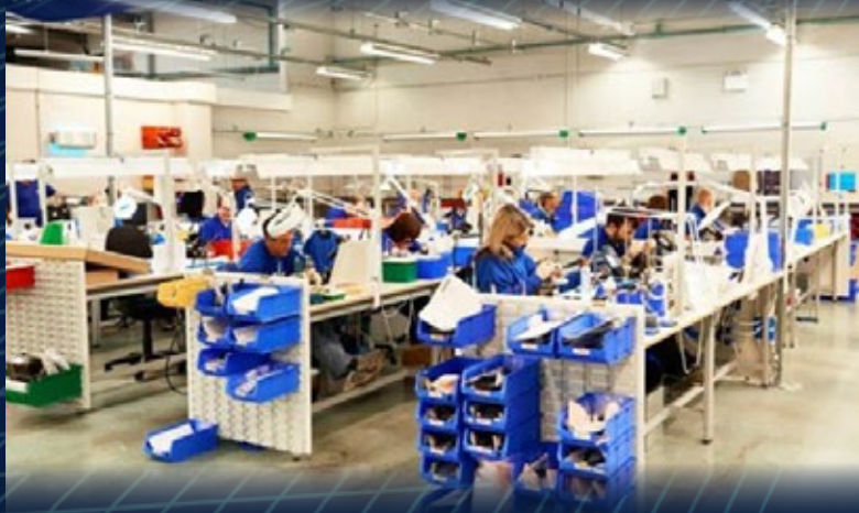
Micro-D and Nanominiature harnessing is completed in our ISO 9001:2008 and BS EN 9100:2003, BS EN 9120:2005 certified facility
