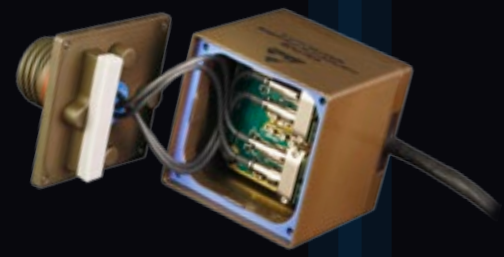
Small form-factor ruggedized opto-electronic media converter
